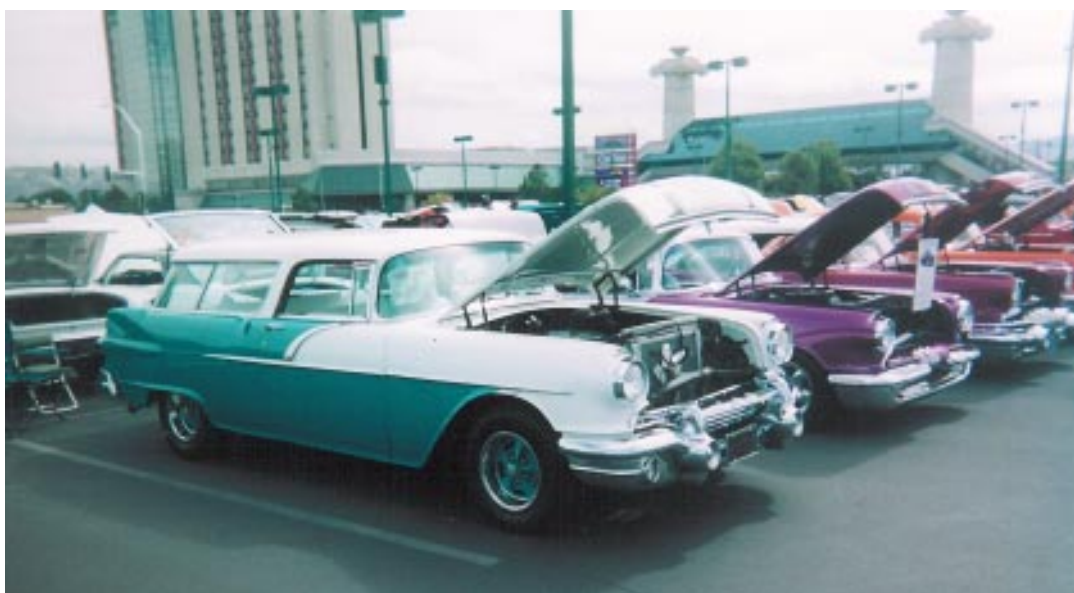
Above: Larry & Debbie Strain's 1956 Modified Safari. It's Turquoise and White and equipped with a '76 Trans Am front clip, a 403 cu. in. engine, 350 Turbo-Hydromatic transmission, and a Trans Am Positraction rear-end.
