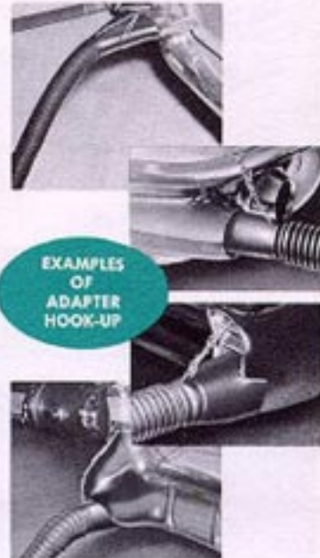
J 6780 Neoprene "Y" Connector Shown With Adapters And J 6781 Hose Cut For Dual Exhaust Adaptation
