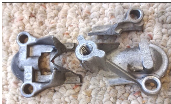
Above: A cracked manifold due to over torqueing. They usually fail after they start of cracking. It does not take much to destroy one so be careful folks!
