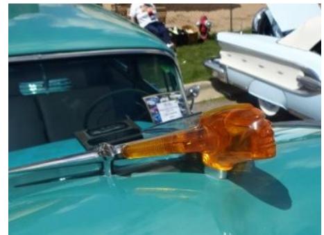
Above Left: The Walkenshaw's aged-cracked hood ornament. Center: Carolyn learns about an old car dealer trick; she applies motor oil to the plastic which quickly makes the cracks nearly disappear. Right: The ornament looks like new after it's first bathing of motor oil. Carolyn now has the duty of keeping her favorite hood ornament looking fresh.
