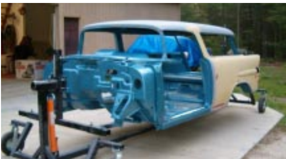
Interior and exterior painting in progress
