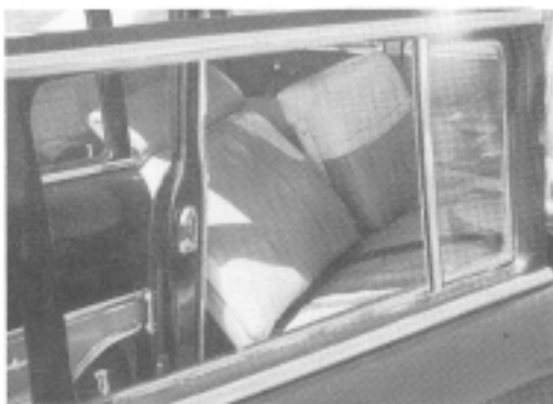
The reclining front passenger seat with folding headrest was a feature ahead of its time.
