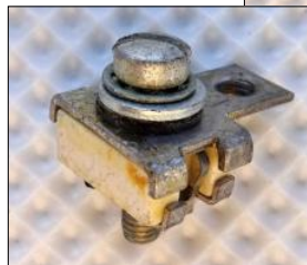
You can find various regulator fuses including Delco. Look for one that covers 25 amps or 30/35 amps for those with factory equipped AC.
