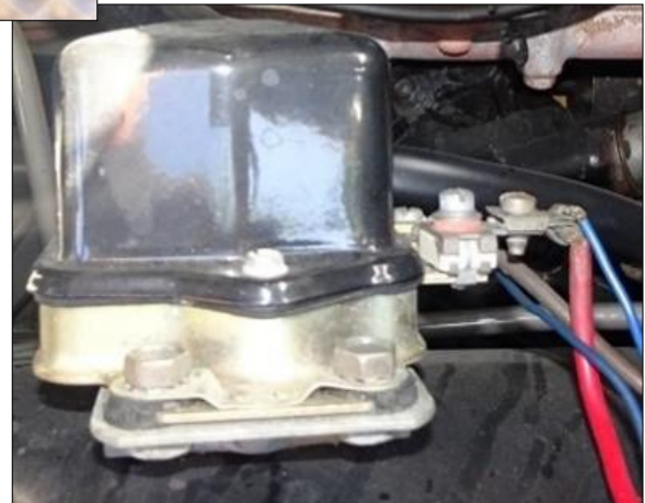
You can find various regulator fuses including Delco. Look for one that covers 25 amps or 30/35 amps for those with factory equipped AC.
