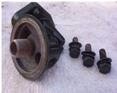
Housing and bolts cleaned, painted & ready for installation
